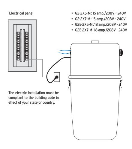
If you experience voltage surge problems on your electrical circuit in spite of adequate connections, a high magnetic circuit breaker can be installed on your electrical panel. Contact an electrician for more information.
