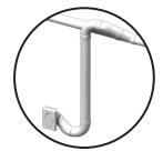
In the basement (connected under a pipeline under the floor)
