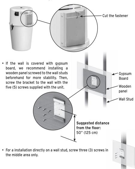
• Lift the head to slide its support onto the wall bracket.
