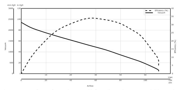
\* Data represents performance of a typical motor sampled from a large production quantity. Individual motor data may vary, due to normal manufacturing variations."
