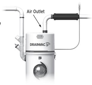
If your model includes 2 motors, the air outlet is on top of the unit. If it only includes 1 motor, the air outlet is on the side of the unit.
